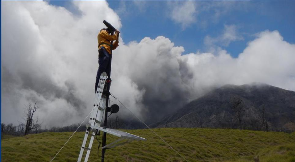
Dr. Maarten de Moor performing maintenance on one of the NOVAC DOAS scanners installed at Turrialba that OVSICORI uses to monitor SO<sub>2</sub> emissions in real time.
